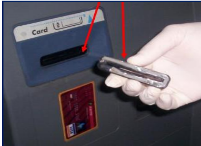
Skimming device placed over Card Reader
