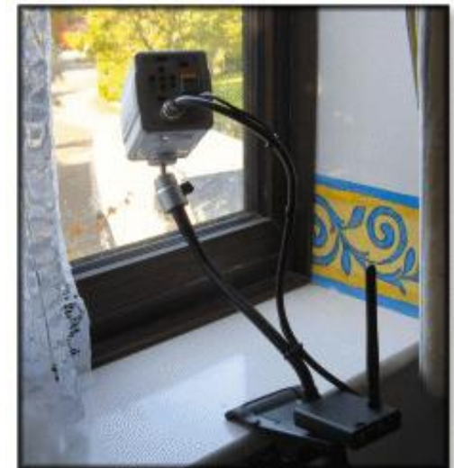
Observation camera across road recording & transmitting PINs
