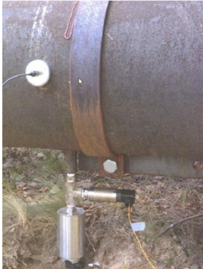
Figure 5: Embedded Robust Sensors on Pipeline
